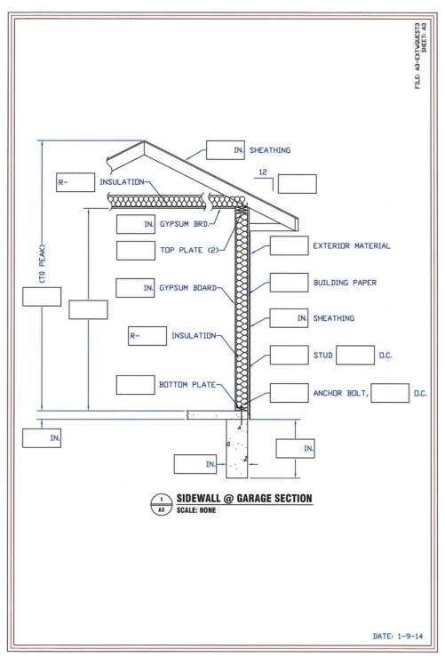
Attachment A3: Sidewall @ Garage Section
