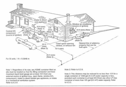
FIGURE 1.1(b) Aboveground ASME Containers. (This figure for illustrative purposes only; code shall govern.)
