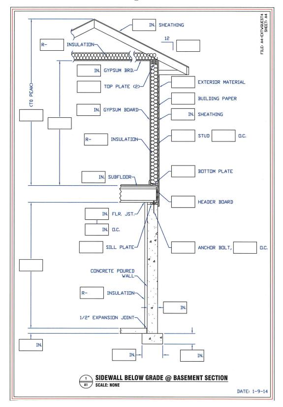
Attachment A2: Sidewall @Walk Out Basement Section
