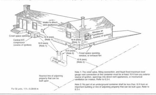
FIGURE 1.1(c) Underground ASME Containers. (This figure for illustrative purposes only; code shall govern.)
